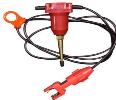
Geophone with cable
