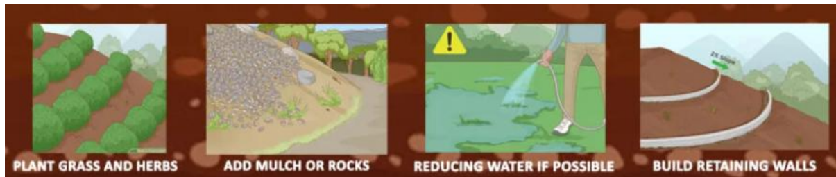
Figure 7.1: Preventive Measures to prevent Soil Erosion/Degradation
