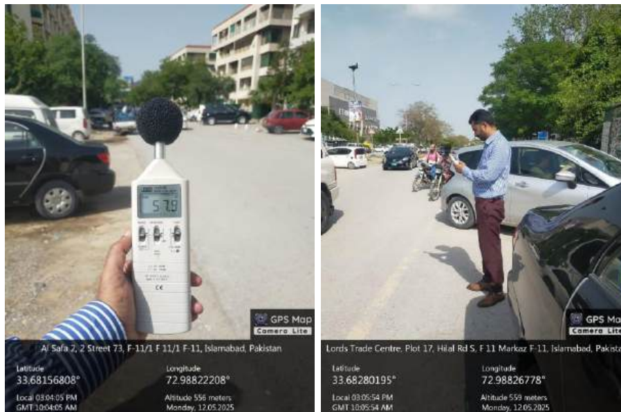
Figure 4.10: Noise monitoring at project site (left) Hilal road F-11/1 Markaz (right)
