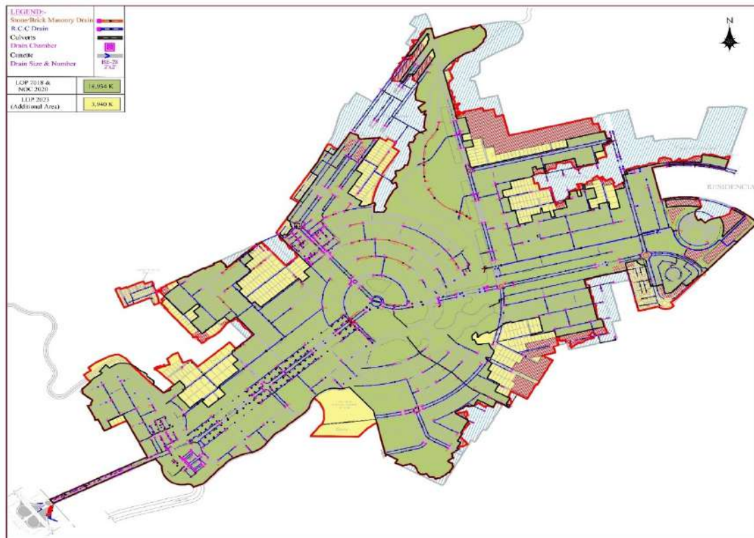
FIGURE 3-10: STORM WATER DRAINAGE SYSTEM
