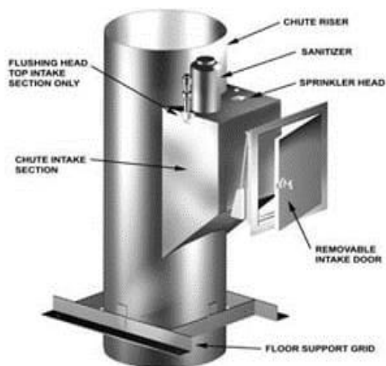
Figure 8.2: Typical Garbage Chute
