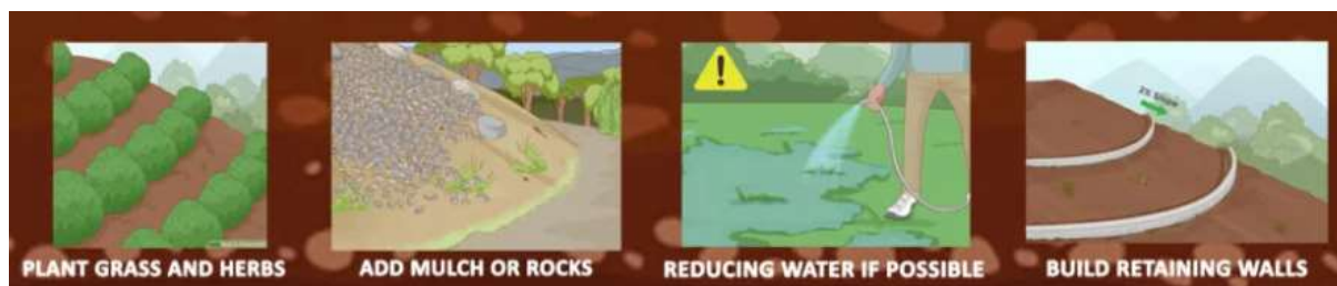
Figure 7.5: Preventive Measures to prevent Soil Erosion/Degradation
