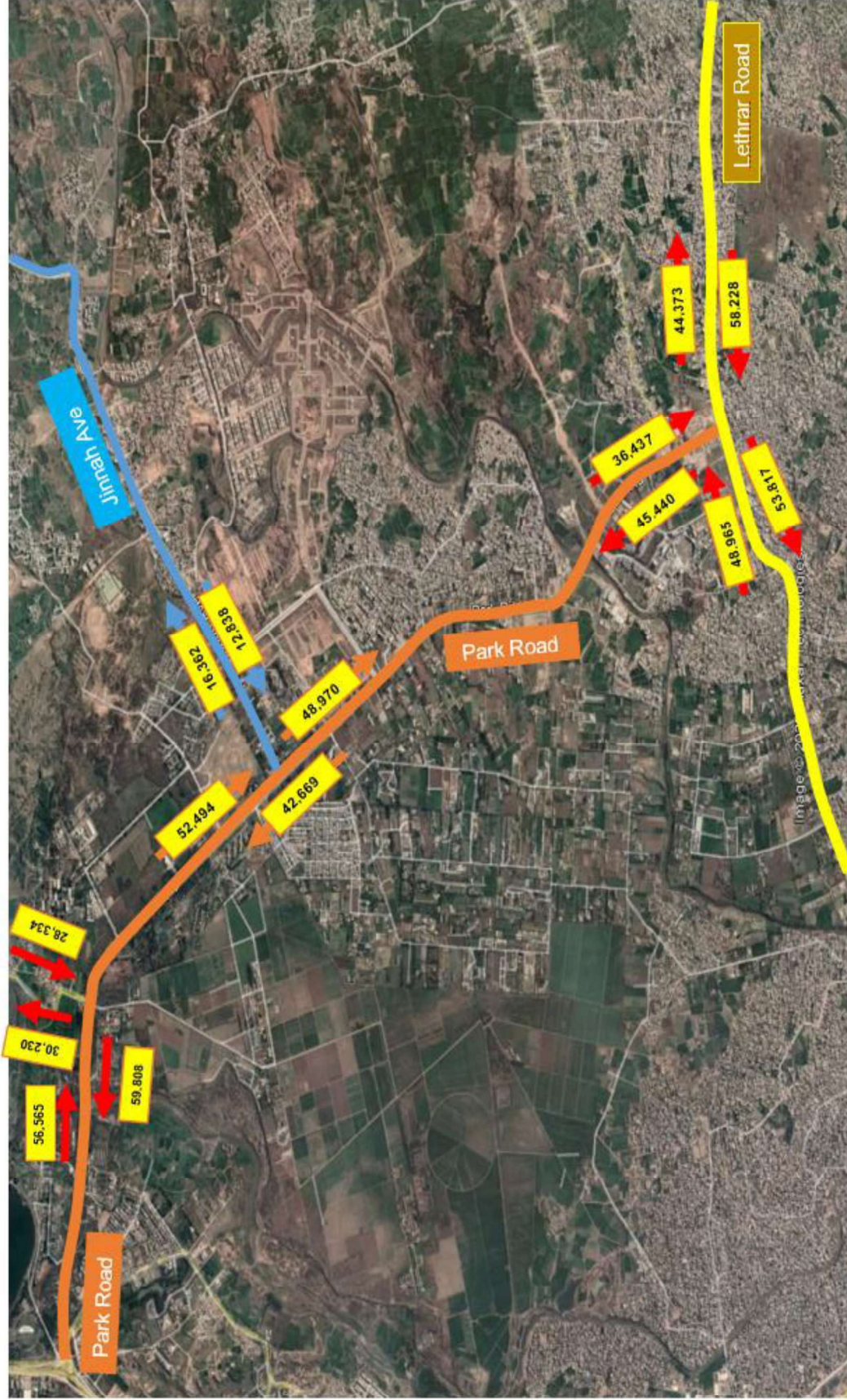
Figure 2-5: Existing Daily Traffic on Current Road Network (2022)
