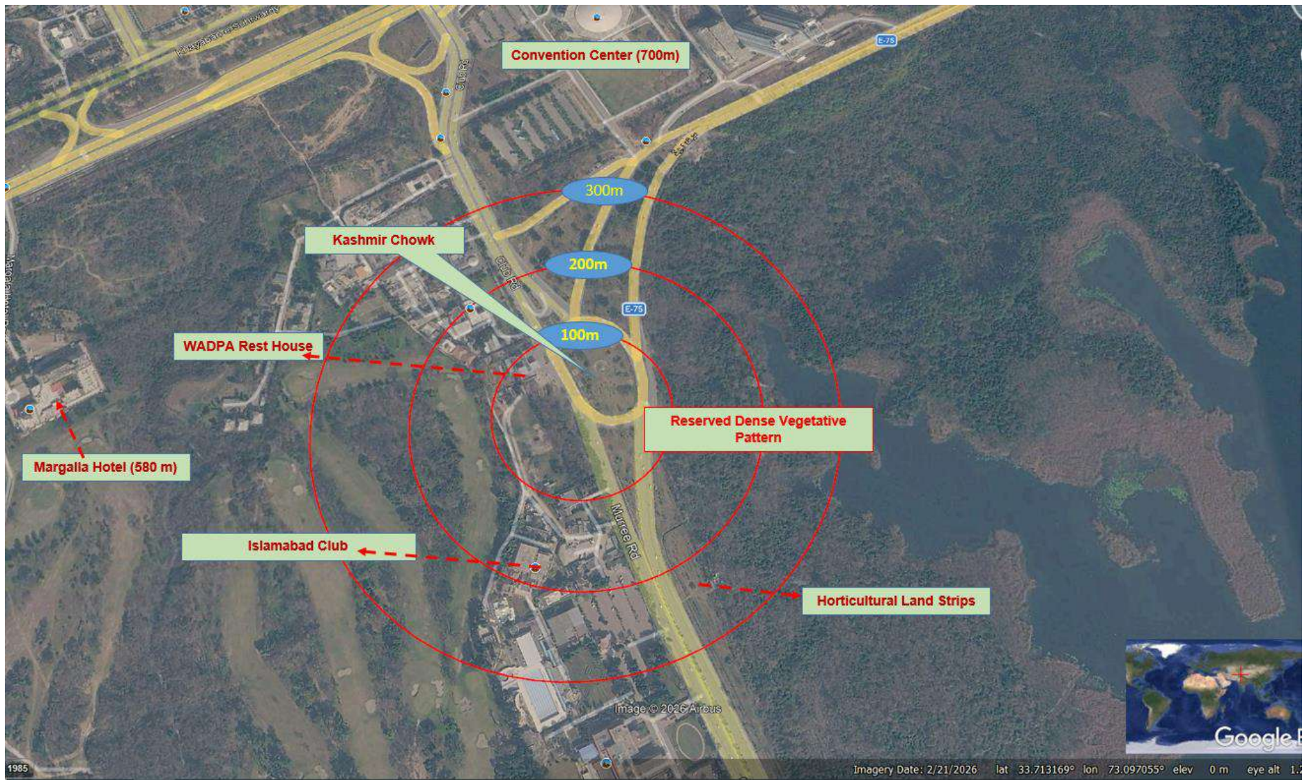
Figure 19: Identified Areas more Susceptible to Affect during Underpass Construction Intervention within Radius of 100, 200 and 300 meter
