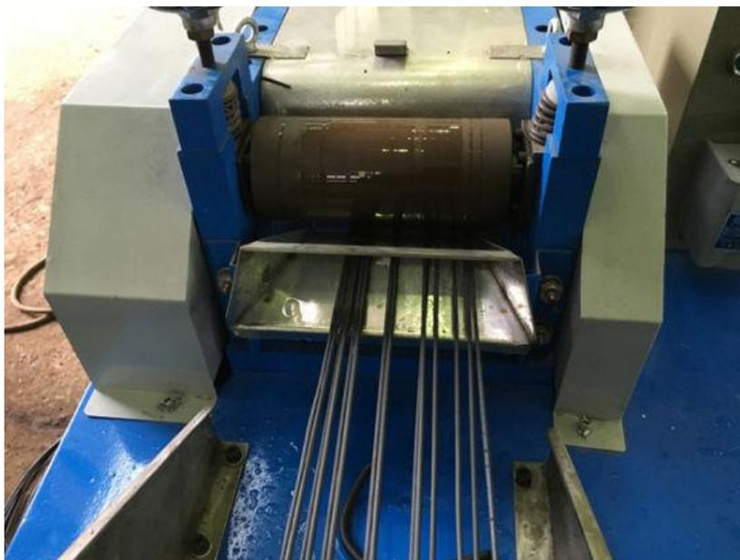
**Image 5 showing cutter machine used for cutting plastic threads into granules**
